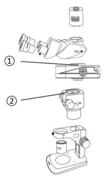
As shown in the figure above, separate the microscope trinocular head from the body, install the fluorescence module in the middle, and then
