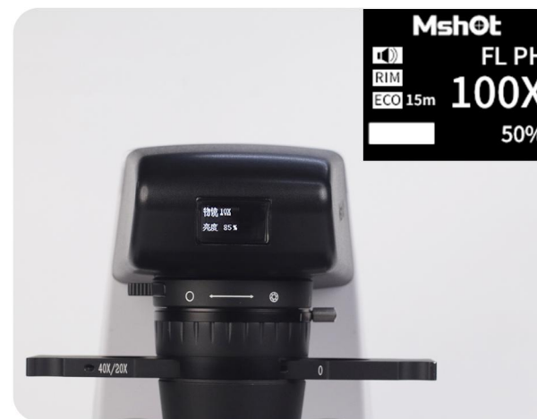
Digital display screen prompts the objective lens magnification and light intensity
